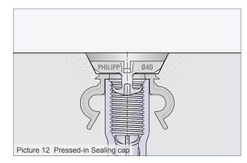
Then, the Plastic sealing cap can be unscrewed easily.
