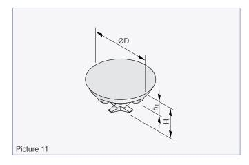
Sealing caps are used exclusively as visual attractive closing of the recesses. In order to avoid damage to the concrete element (e.g. spalling due to frost), the user shall ensure that the Sealing caps are protected against moisture penetration.
